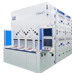
Backside Clean Tool for wafer device side none contact process
