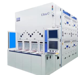
High Temp IPA Drying for advance Logic processes
